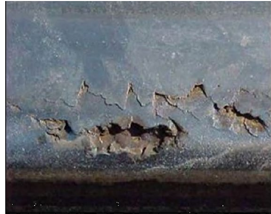
Close Up of Flaking on Gage
