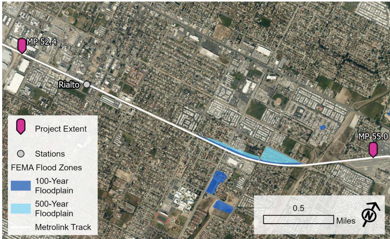
Figure 39: Project Area Map and Flood Exposure, Lilac to Rancho Double Track Project
